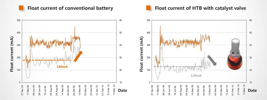
Under elevated operating temperature (above 40°C), the float current and temperature of 12V100Ah conventional monobloc is much higher than the one that is equipped with catalyst valve in each cell
