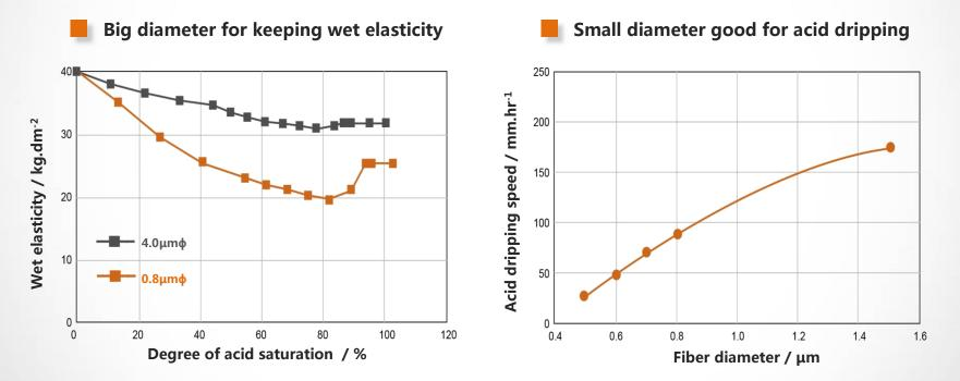
The diameter of fiberglass on separator is an important factor: bigger diameter is good for keeping wet elasticity, while smaller one is good for acid dripping. We found most rational proportion by many tests
