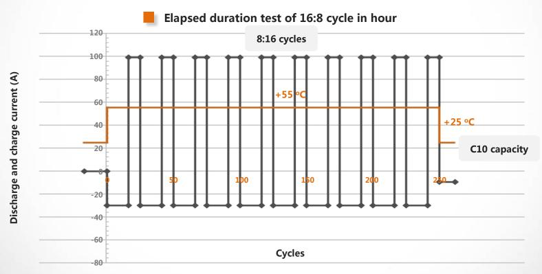
Test condition: under 55 degrees, 80% DOD, and recharge time of 8 hours
