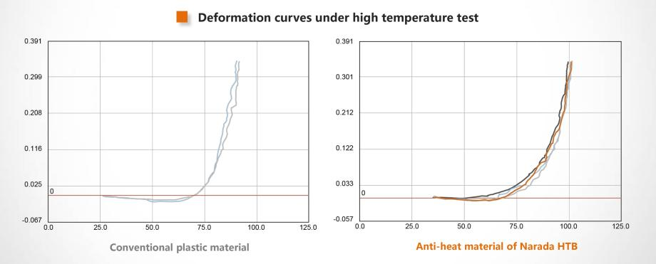
Innovative case material of HTB battery against high temperature (Patent of invention: 200810059699.3)
