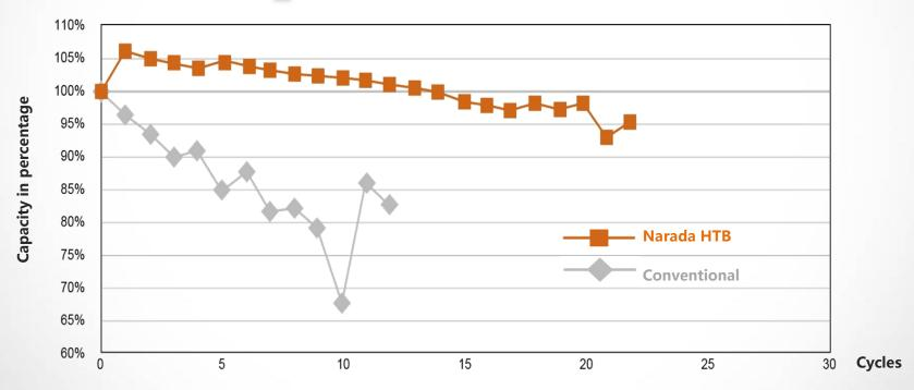
Note: The batteries have been tested for 10 months (20 daily discharge cycles and 21 times residue
