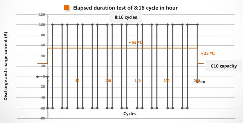
Test condition: under 55 degrees, 80% DOD, and recharge time of 16 hours
