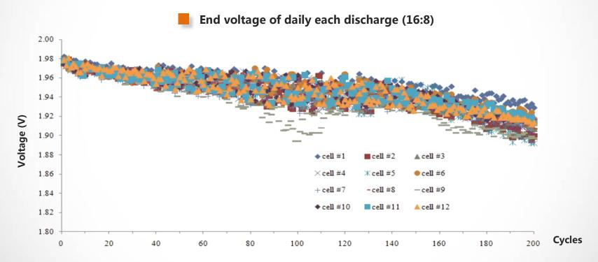
Note: The batteries have been tested for 10 months (20 daily discharge cycles and 21 times residue capacity determination) by InterTek Test Report – An international recognized authority of the 3rd party
