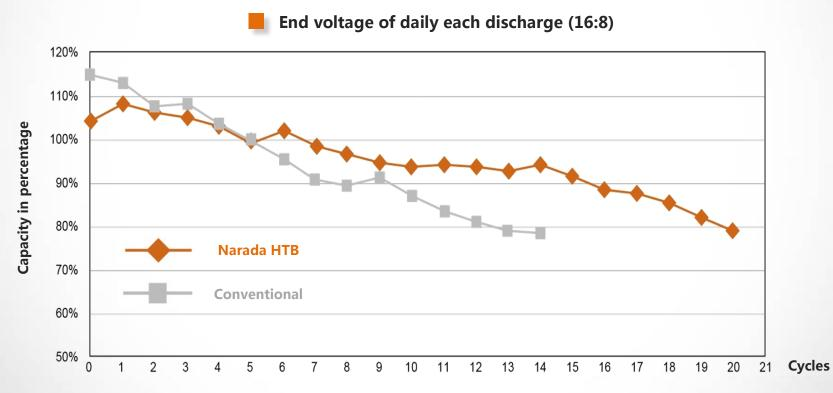
Note: The batteries have been tested for 10 months (20 daily discharge cycles and 21 times residue
