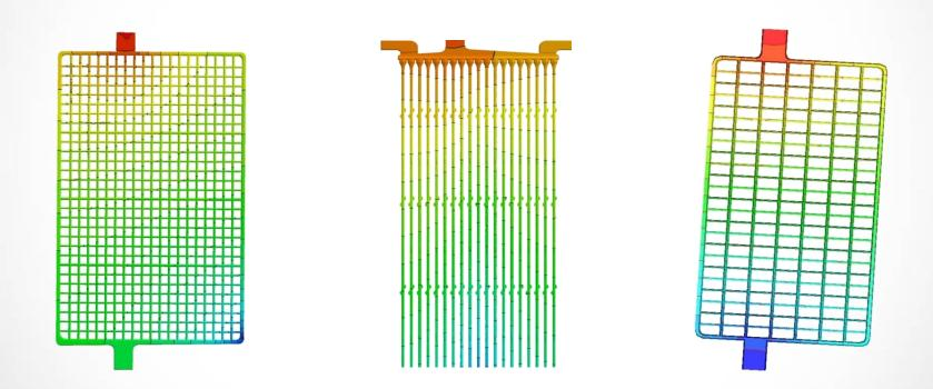
The structural design of positive plate has been modified and adapted in thickness in order to achieve lower a lower Pavlov  $\gamma$  factor, so that the cyclic performance and charging acceptance can be improved
